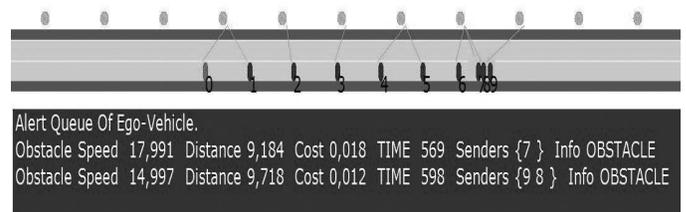
Fig. 5. Ego-vehicle receives through the Road Infrastructure messages reported by I-WAY vehicles with id numbers 7, 8 and 9.
