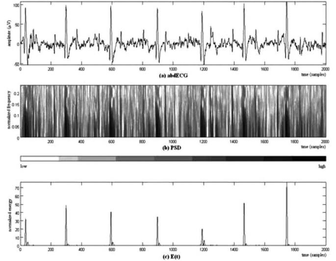
Fig. 3. Time–frequency analysis. (a) abdECG signal, (b) PSD of the abdECG signal, and (c) energy distribution versus time.
