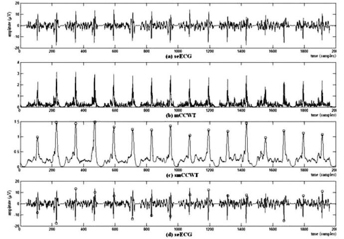
Fig. 6. Wavelet analysis and candidate fetal R-peak detection. (a) seECG signal, (b) modulus of the CCWT coefficients (mCCWT), (c) smoothed modulus of CCWT coefficients (smCCWT) and detected peaks (circles), and (d) seECG signal and candidate fetal R-peaks (circles).
